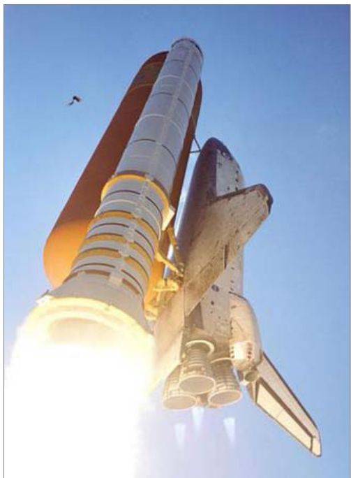
In the wrong place at the wrong time, a bird is silhouetted against the clear blue Florida sky (upper left) as it falls away from Space Shuttle Discovery after hitting the external tank during liftoff of mission STS-114 in July 2005. NASA hopes an avian radar detection system will help avoid such strikes in the future. Image credit: NASA
