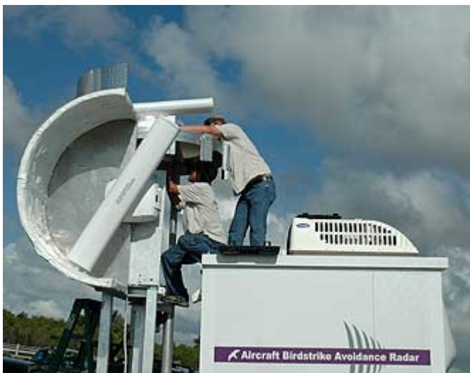
The avian radar in position at Launch Complex 39 offers the ability to monitor either of the two shuttle launch pads during a countdown. Technicians adjust the system's two customized marine radars that provide both horizontal and vertical scanning. Image credit: NASA
