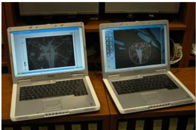
Inside the Launch Control Center at NASA's Kennedy Space Center, data relayed from the avian radar (right laptop) aided by camera images (left laptop) will help controllers recognize when any large birds are in dangerously close proximity to the vehicle and hold the countdown when necessary. Image credit: NASA
